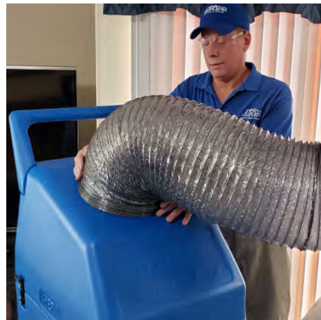
3. Connect a 12” hose to the 12” TurboJet inlet.
