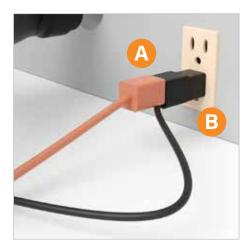
5) Plug the drill into the foot pedal switch (A) and plug the pedal cord into the wall (B). Press the Drill's Trigger and lock it in the "ON" position. It will only run when the foot pedal is pressed. The pedal leaves both hands free.
