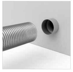
2) Turn off the dryer, remove power, then move it away from the wall and disconnect the exhaust tubing. If it is a gas dryer, be careful to not damage or break the gas line.
