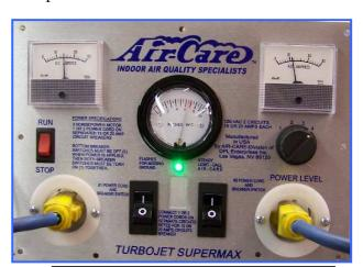
Panel shows with "GREEN" status Light, 2 power cords connected, Power Level #4 (3 HP), Running (6" Static Pressure)
