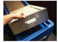
3. Use care when removing the 3<sup>rd</sup> stage HEPA filter mounted in the bottom half of the cabinet. When the airflow through the inlet is noticeably reduced and the 1<sup>st</sup> & 2<sup>nd</sup> stage filters are clean, it is time to replace the 3<sup>rd</sup> stage HEPA filter.
