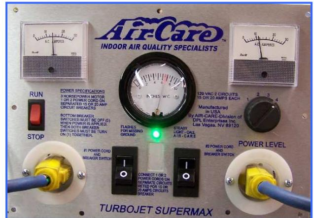
Panel shows with “GREEN” status Light, 2 power cords connected, Power Level #4 (3 HP), Running (6” Static Pressure)
