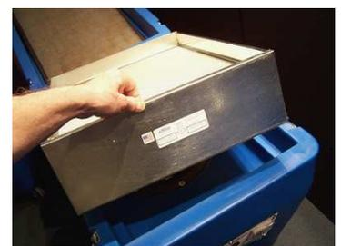
**NOTE:** Applying compressed air pressure or using a vacuum brush on filter surface will damage the filter. If you have any questions regarding the HEPA filter maintenance, please call Air-Care at 800-322-9919
